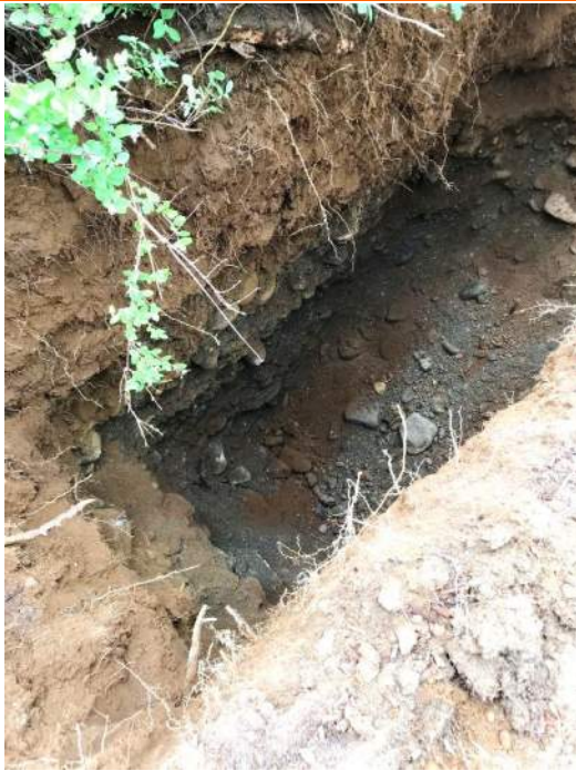
Cobbles and Boulders (TP-18)
