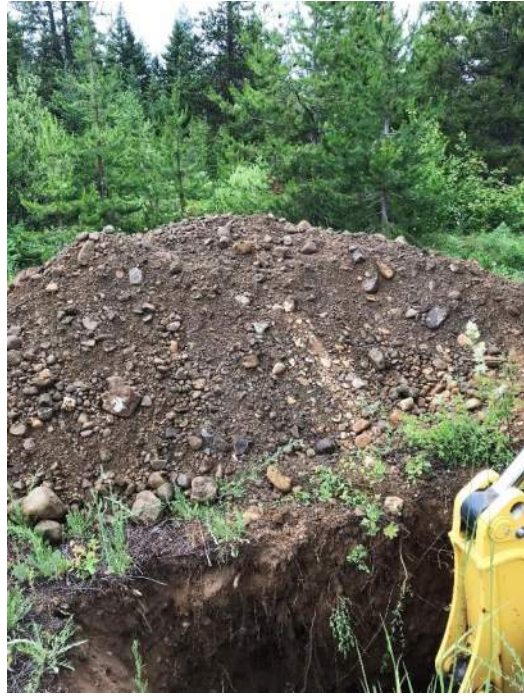
Cobbles and Boulders (TP-5)
